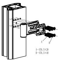
6. Adjust as necessary. It may be necessary to slacken sash screws whilst carrying out lateral adjustment. Re-tighten screws, secure front cover and fit top cover and screw cover.
