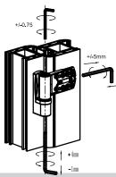
5. When all hinges are fitted slide sash onto frame. Fixing cover plate with screw (retained in plate)
