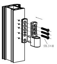
3. Firmly push hinge pin into place (with pin in neutral position to allow +/- 0.75mm adjustment noting offset position) then slide gap cover over pin
