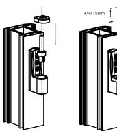
4. Fit flag to sash using screws supplied (28mm through 1st position & 40mm into main chamber)
