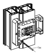
2. Add packers if required then fit hinge body usng 40mm screws (supplied)
