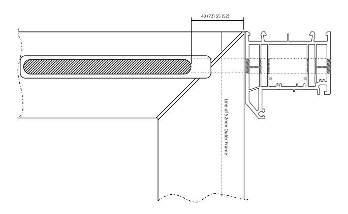
Link Vent 2500 overall width = 236mm (Min Frame Width = 314mm)
